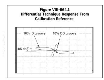
standard discontinuities. The responses shall be clearly indicated by the instrument and shall be distinguishable from each other as well as from probe motion signals.
